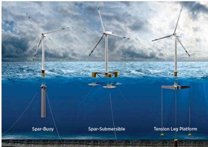
Figure 5.3: Sample of floating foundation designs
