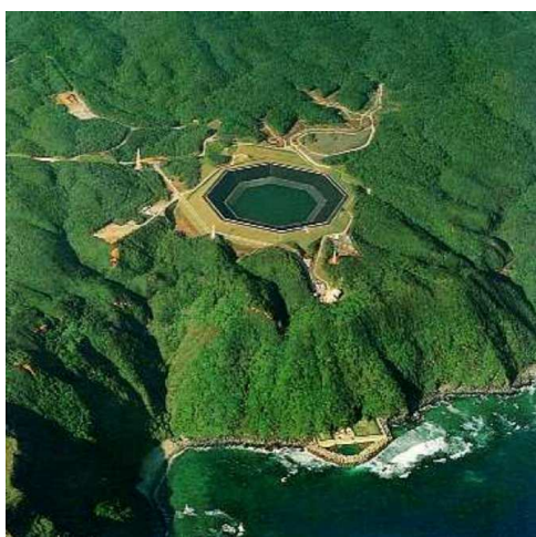
Figure 5.5: Yanbaru Okinawa pumped hydro energy storage
