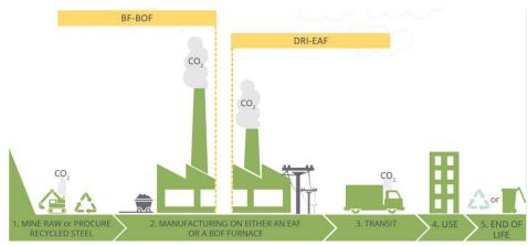
Based on (4). Note: BF = blast furnace; BOF = basic oxygen furnace; CO<sub>2</sub> = carbon dioxide; DRI = direct reduced iron; EAF = electric arc furnace.
